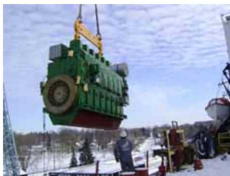
Above: Setting the new port MAK diesel, December 2009.
