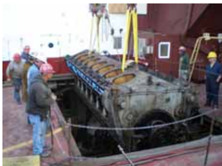
Above: Starboard Pielstick removal, November 2009.
