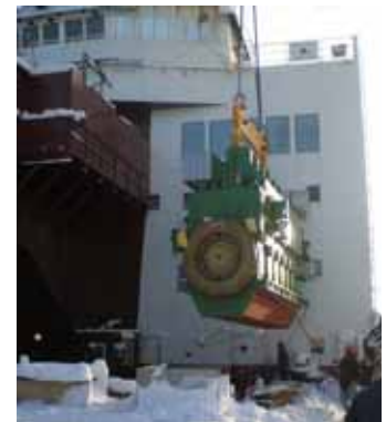
Above: Setting the new port MAK diesel, December 2009.
